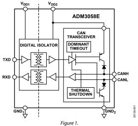
regulatory approvals (pending) for a 5.7 kV rms withstand voltage and a 1500 V peak working voltage ensure that the ADM3058E meets application isolation requirements.
