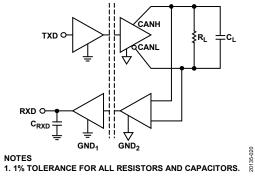
Figure 19. Switching Characteristics Measurements
