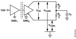
Figure 17. Driver Voltage Measurement
