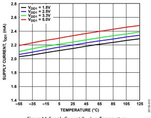
Figure 14. Supply Current (I<sub>DD1</sub>) vs. Temperature
