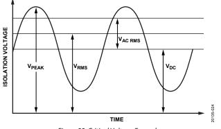
Figure 23. Critical Voltage Example
