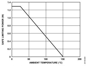
Figure 4. Thermal Derating Curve, Dependence of Safety Limiting Values with Ambient Temperature per DIN V VDE V 0884-11 (See the Thermal Resistance Section for Additional Information)
