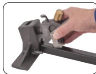
Screw the rectangular gauge adapter nipple into the thread of the pressure gauge tightly, so that a good seal is formed. Make sure the flat surfaces of the nipple are aligned with the pressure gauge.
