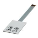
Membrane keypad for BC 107,6 and BC 161,6, self-adhesive, conductive silver technology, 4 keys, 2 colors, 7-pos. terminal lug, pitch: 1.0 mm, customizable in the online configurator
