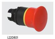
Head position visible from the side with yellow collar Compliant with the requirements of emergency stop: IEC 60947-5-5 /EN 418/ISO 13850
