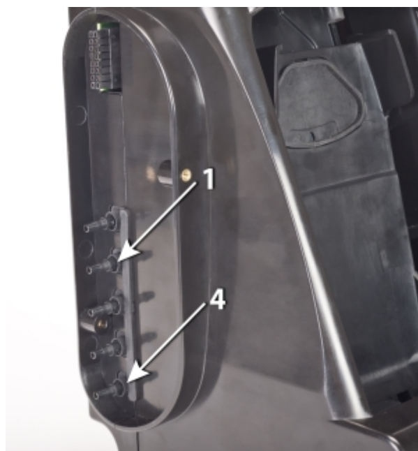
Figure 15 Gas inlets on the Test Stand
