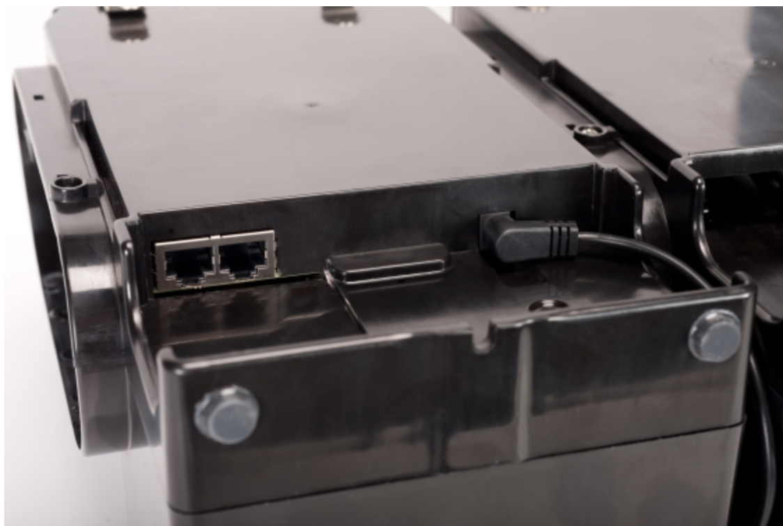
Figure 5 Test Stand Ethernet jacks
