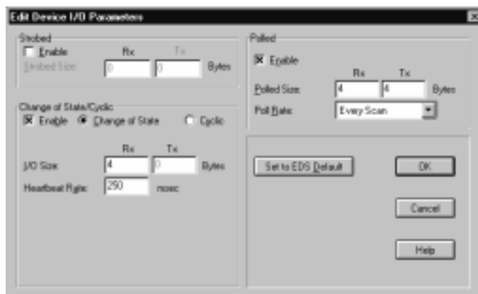
Figure B.6 Edit Device I/O Parameters Dialog Box for Polling and COS
