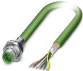
Bus system flush-type plug, INTERBUS, 5-pos., M12, shielded, B-coded, rear/screw mounting with M16 thread, with 5 m bus cable, 3 x 2 x 0.25 mm 2
