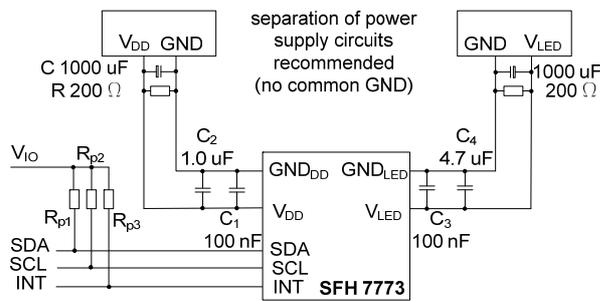
Fig. 17: Suggested setup for evaluation of the SFH7773 in a laboratory environment. R and C improve the dynamics of the power supply. C<sub>1</sub> and C<sub>3</sub> should be placed next to the respective supply pins (same for C<sub>2</sub> and C<sub>4</sub>). Special considerations should be paid to separate the supply circuits (V<sub>DD</sub> and V<sub>LED</sub>).
