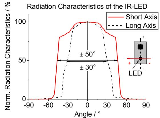
Fig. 10: Radiation characteristics of the proximity sensor LED.
