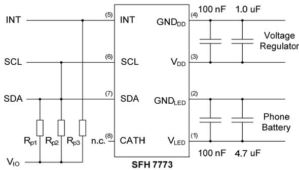
Fig. 19: Recommended implementation into a mobile phone environment.
