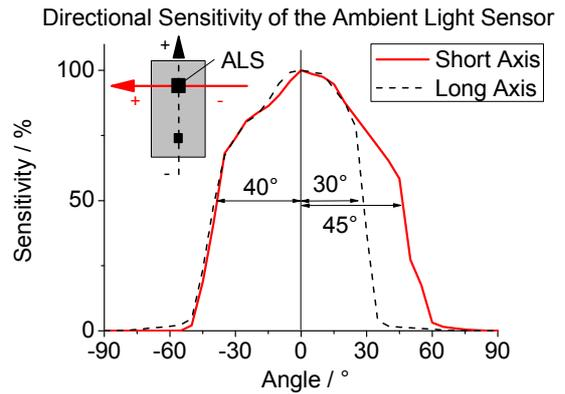
Fig. 5: Directional characteristics of the ambient light sensor.
