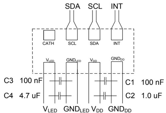
Fig. 18: Layout suggestion for a single sided pcb: The power supply circuits must be decoupled to achieve a low noise operation of the PS with high LED drive current. C<sub>1</sub> and C<sub>3</sub> need to be placed next to the respective pins (as well as C<sub>2</sub> and C<sub>4</sub>).
