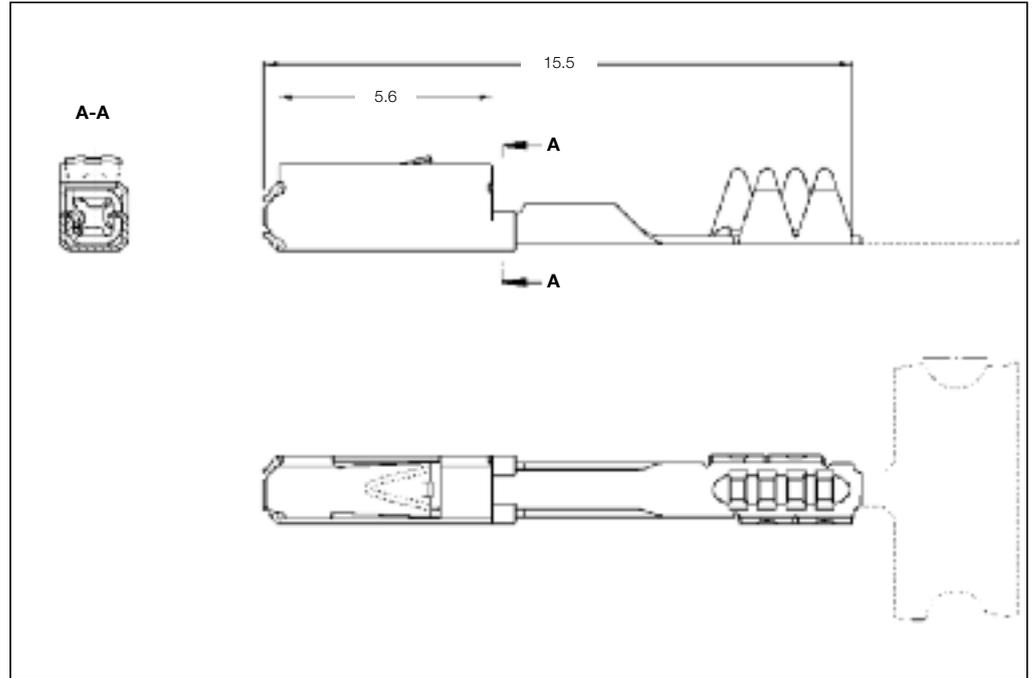
**MQS Flexible Flat Cable (FFC) Receptacle Contacts**
