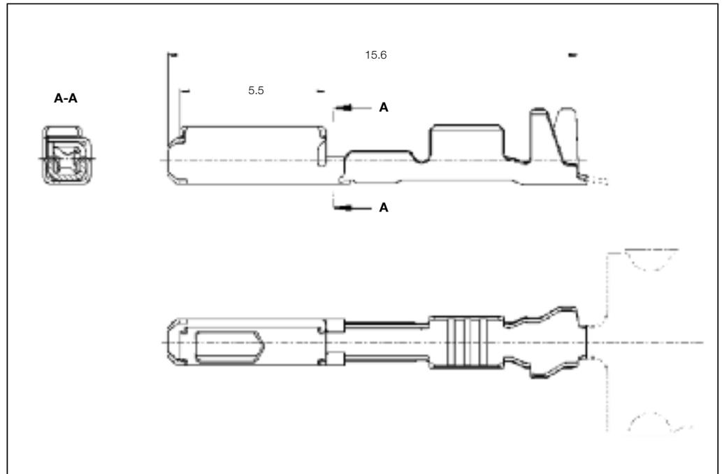
**MQS Clean Body Receptacle Contacts with Short Circuit Area**
