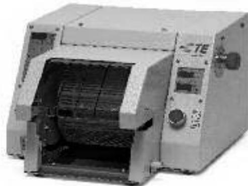
In this way the operator is able to efficiently load both machines and so minimise 'dead time'. Installing Raychem splice sealing products immediately after welding gives reduced installation time and earliest possible mechanical protection for the welded joint. The operator positions the splice sealing product centrally over the splice joint and then locates the assembly into the gripper mechanism.
