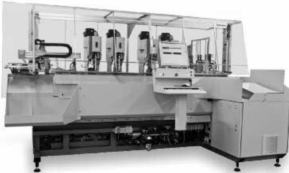
Together, the Zeta 633 and Zeta 651 harness makers offer a reliable and attractively priced complete solution for the single-sided loading of single and double row blocks.
