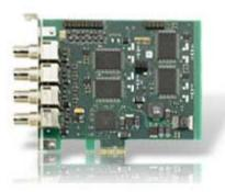
The pciGrabber-4x4 offers up to four fully independent input channels, each with its own video decoder.
