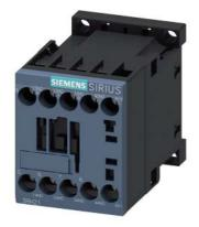
Coupling contactor relay, 4 NO, 24 V DC, 0.85 ... 1.85\* US, with integrated diode, Size S00, screw terminal
