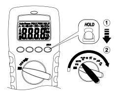
Dial the switch to off position ,then keep the HOLD button down and turn the meter on.
