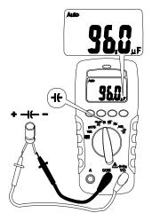
Dial the switch to select the measuring function.
