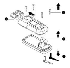
Fuse type: 11A/1000V - 20KA (10x38mm)
