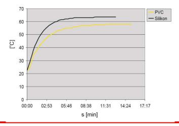
PVC - reaction to air temperature from 22.5 °C .. 58 °C (from 72.5 ..136.4 °F).
