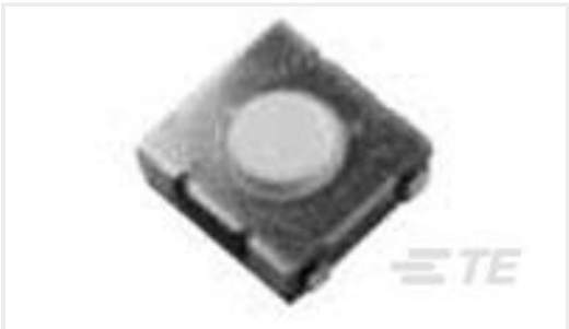
TE Part #1571636-8 TACT,SMT,GULL WING,160GF,T&R
