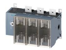
Switch disconnector with fuse 800 A, Size 5, 3-pole for LV HRC fuse Sz. 2 and 3 Front operating mechanism left Basic unit without handle flat terminal
