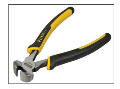
FatMax end cutting plier with bi-material handles and heat treated chrome steel forging. Has an interlocking joint assembly and high frequency heat treated cutting edges. It is ideal for very close cropping of wire to the surface of the workpiece.
