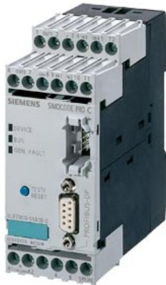
UNIDAD BASE 1 SIMOCODE PRO C INTERFAZ PROFIBUS DP 12 MBAUDIOS, RS485 4E/3S PARAMETRIZABLE US: DC 24V ENTRADA PARA CONECTAR TERMISTOR SALIDAS MONOESTABLES
