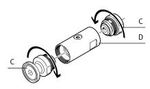
Tighten both covers (C). Observe tightening torques (→ Chapter 8).
