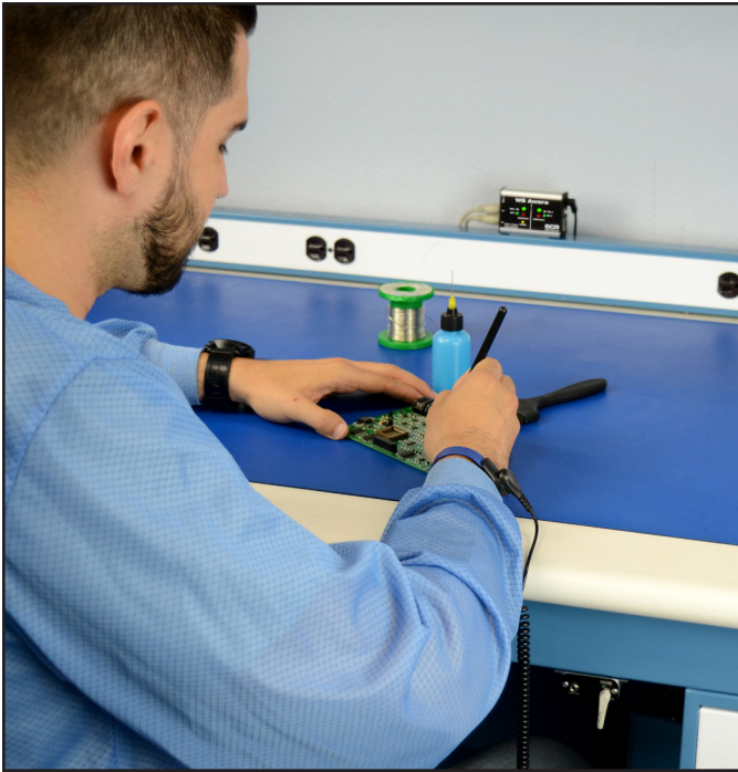
Figure 13. Using the 770067 WS Aware Monitor on a workbench
