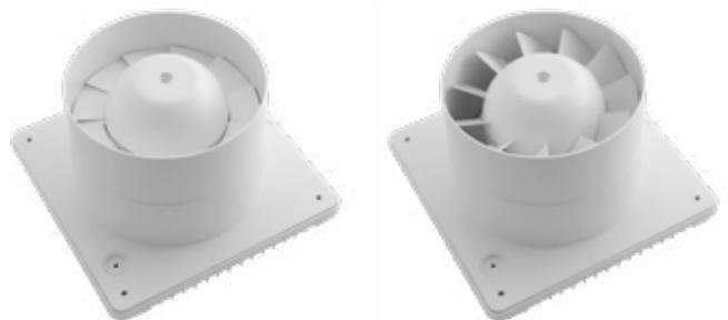
The EDM's electric shutters operate using wax motor technology. The wax pot is a paraffin-filled cylinder designed to open and close the shutter with a smooth and gentle stroke. This reduces noise and ensures faultless operation every time.
