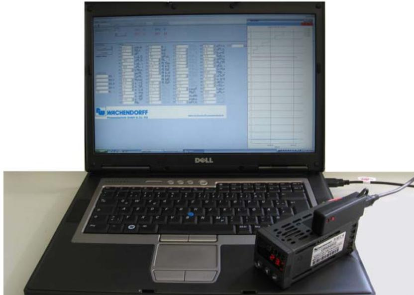
Figure 1: Wachendorff Software with Programming module
