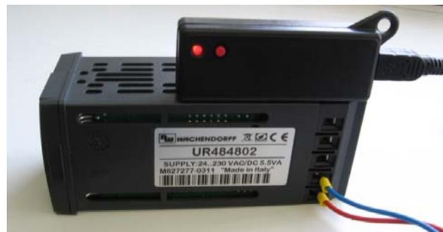
Figure 3: Inserting Programming module on UR4848xx
