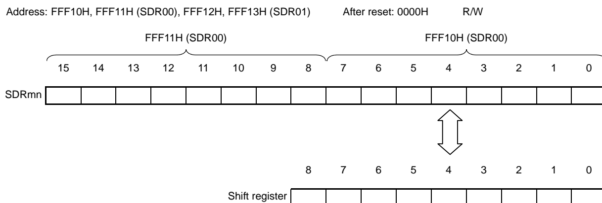
Figure 14 - 2 Format of Serial data register mn (SDRmn) (mn = 00, 01)
