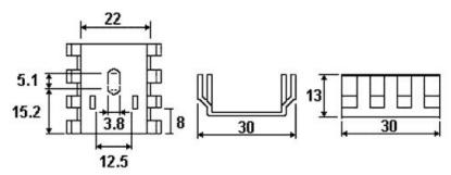
DEVICE MAY BE FITTED WITH SCREW OR CLIP (CLIP 04)
