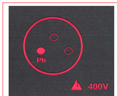
Earth not connected Phase on left Incorrect voltage
