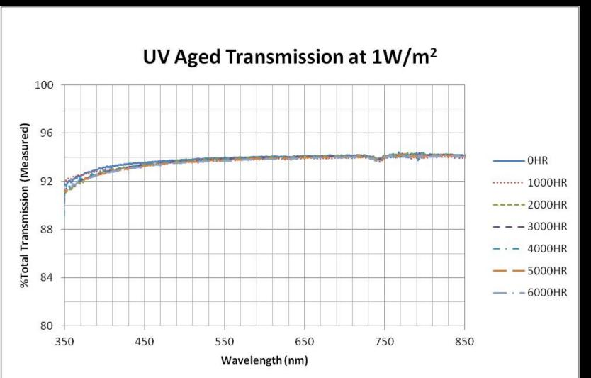
ROSE-UV lenses exposure for heavy UV-radiation over 6000 hours without noticeable change in the transmission.
