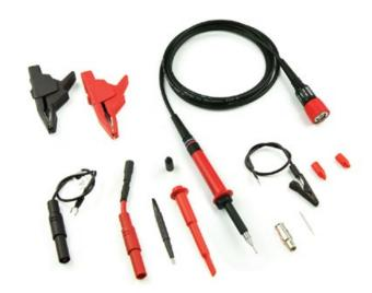
The PPE series includes four fixed-attenuation probes covering a range from 2 kV to 6 kV, and one switchable probe providing  $\div 10/\div 100$  attenuation for voltage inputs up to 1.2 kV. All fixed-attenuation, standard probes automatically rescale compatible Teledyne LeCroy oscilloscopes for the appropriate attenuation of the probe.
