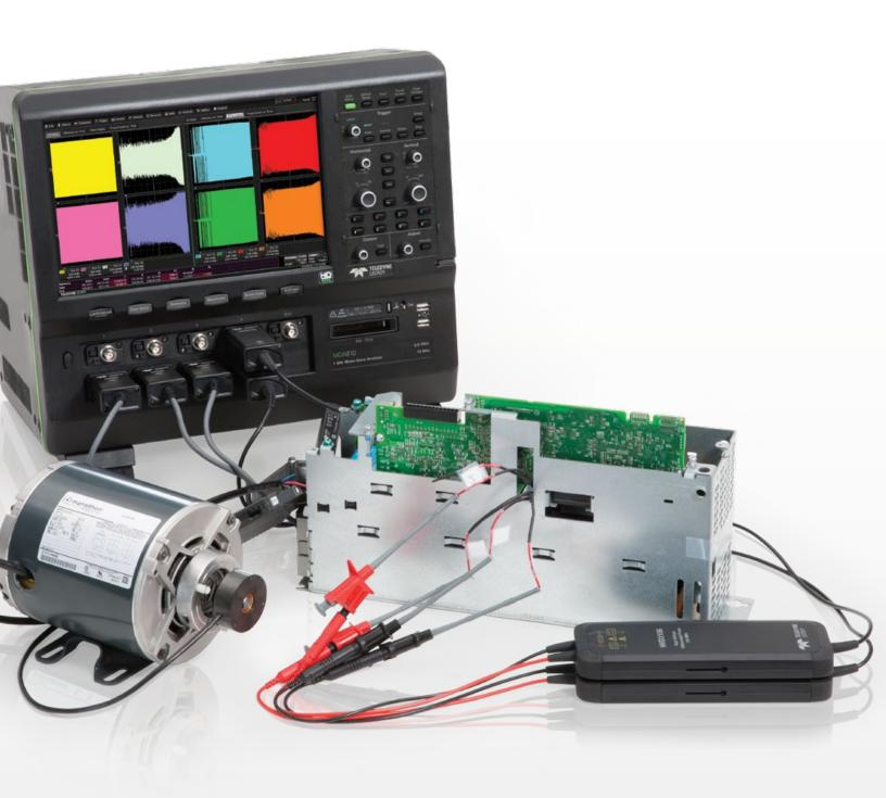
Differential active probes are like two probes in one. Instead of measuring a test point in relation to a ground point (like single-ended active probes), differential probes measure the difference in voltage of a test point in relation to another test point.
