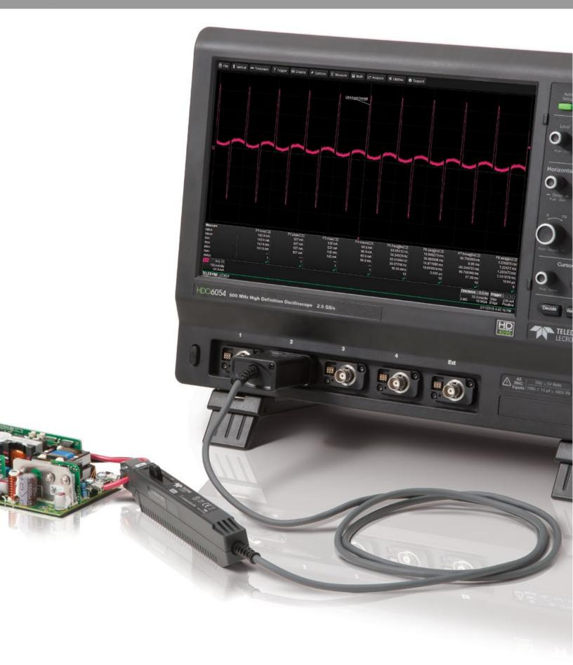
Teledyne LeCroy current probes do not require the breaking of a circuit or the insertion of a shunt to make accurate and reliable current measurements. Based on a combination of Hall effect and transformer technology, Teledyne LeCroy current probes are ideal for making accurate AC, DC, and impulse current measurements.
