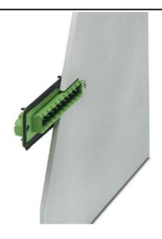
Header, nominal current: 12 A, rated voltage: 250 V, pitch: 5.08 mm, no. of positions: 2, mounting: Soldering
