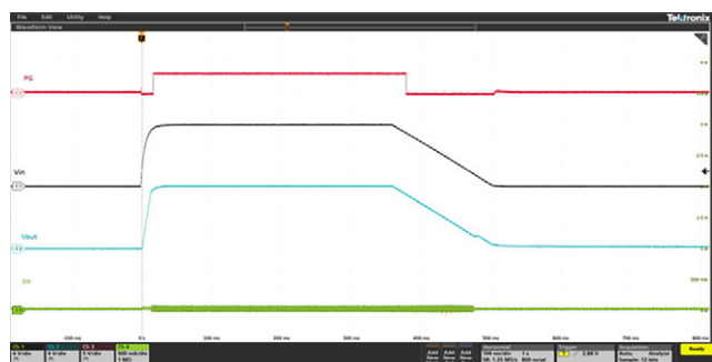
Fig. 20 - Power Up and Down With Input Supply V_{IN} = 22\text{ V} , C_{OUT} = 22\text{ }\mu\text{F} , C_{SS} = 3.3\text{ nF} , V_{EN}/UVLO ramped from 0\text{ V} \rightarrow 12\text{ V} \rightarrow 0\text{ V}
