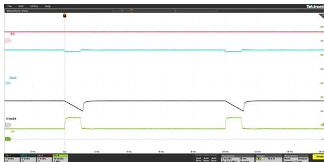
Fig. 30 - Transient Overcurrent Blanking Timer Response V_{IN} = 12 \text{ V} , CITIMER = 3.3 pF, C_{OUT} = 220 \mu F , R_{ILM} = 680 \Omega , I_{OUT} ramped from 7 A \rightarrow 15 A \rightarrow 7 A within 1 ms
