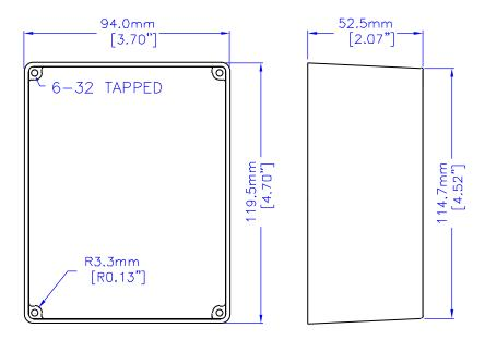
NOTE: FOR DETAIL DIMENSIONING REFER TO DRAWING # 1590C
