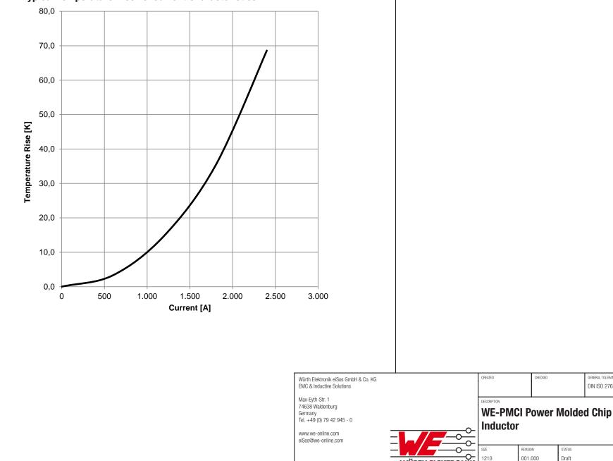
**Typical Temperature Rise vs. Current Characteristics:**
