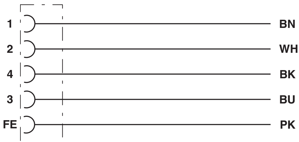
Contact assignment of the M12 socket
