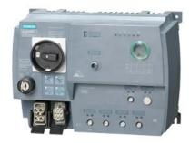
SIRIUS motor starter M200D AS-i Communication: AS-Interface Reversing starter Basic Mechanical switching AC-3, 5.5 kW / 400 V 1.5 A...12.00 A Electronic overload protection Thermistor: THERMOCLICK / PTC with brake contact 400 V AC 2DI AS-i + 2DI / 1DO on device Han Q4/2 - Han Q8/0 with manual on-site operation and key-operated switch
