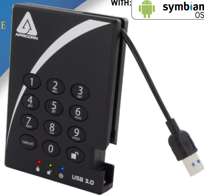
ON-THE-FLY 256-BIT AES-XTS HARDWARE ENCRYPTION
