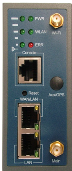
Figure 8. Antenna, Power, Console, LED, LAN / WAN Interfaces
