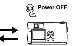
To save battery power, the camera automatically enters the sleep mode after about 3 minutes of non-operation. If the monitor is on, it will automatically turn off. The camera activates again as soon as you lightly press the shutter button or zoom lever. Whenever possible, turn the camera off when you do not intend to take any pictures for a while.
