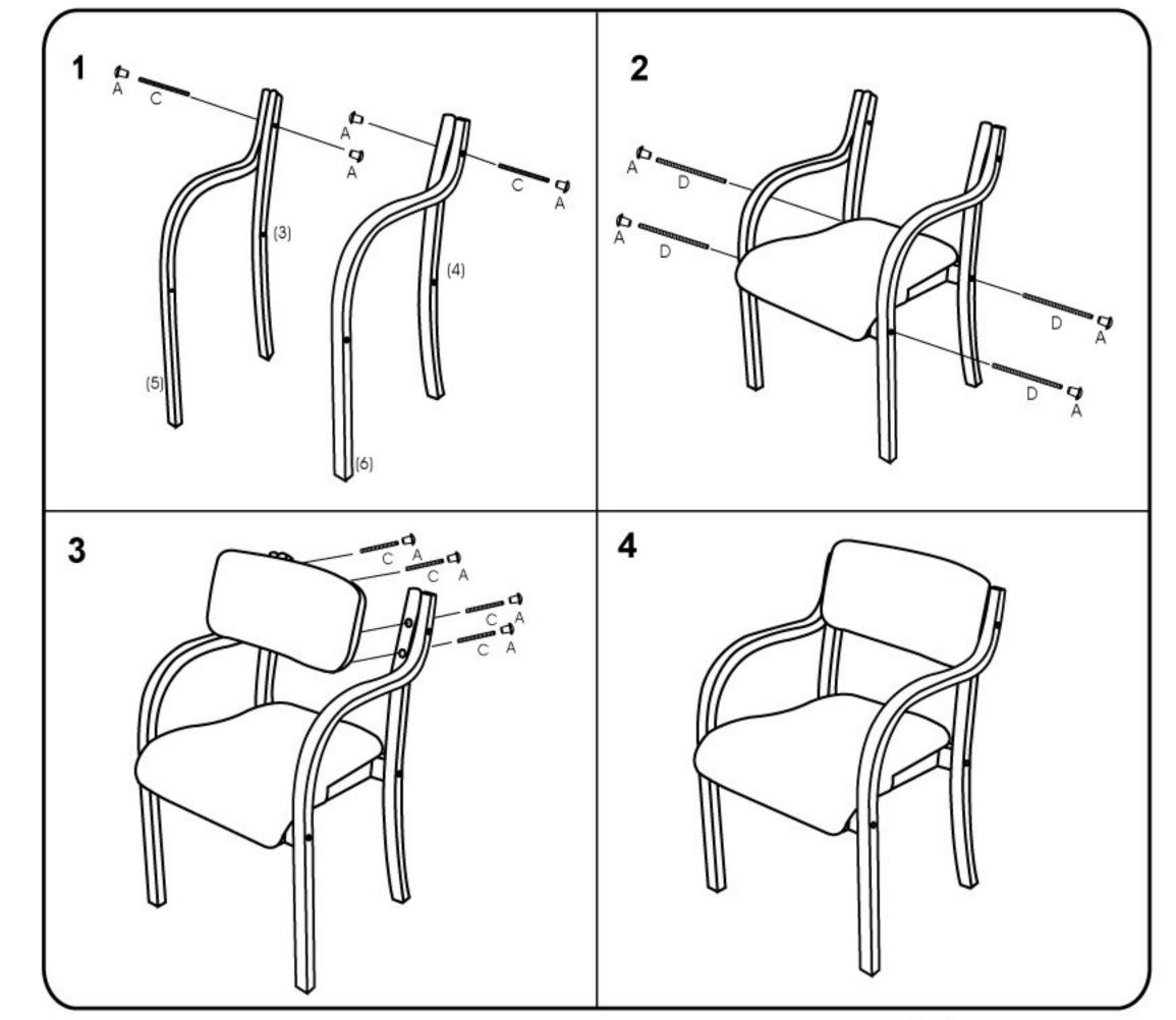
It is important to assemble all parts so that the directional "Arrows" point in the same direction. Make certain that all screws are FULLY tightened before using the chair. Each month, check all screws and tighten any that may have loosened.
