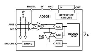
A 2.5 V reference is included onboard, or the user can provide an external reference voltage for gain control or matching of multiple devices. Fabricated on a state-of-the-art BiCMOS process, the AD9051 is packaged in a space saving surface mount package (SSOP) and is specified over the industrial temperature range ( $-40^{\circ}$ C to  $+85^{\circ}$ C).
