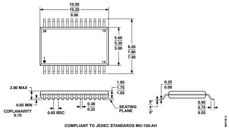
Figure 7.28-Lead Shrink Small Outline Package [SSOP] (RS-28) Dimensions shown in millimeters
