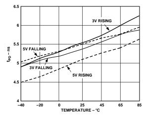
TPC 16. t<sub>PD</sub> vs. Temperature 3 V/5 V
