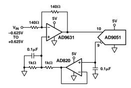
Figure 3. Single Supply, Single-Ended, DC-Coupled AD9051
