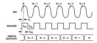
Figure 1. Timing Diagram
