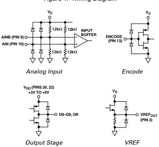
Figure 2. Equivalent Circuits
