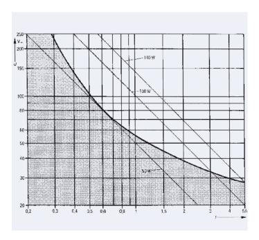
I = switching currentU = switching voltage
