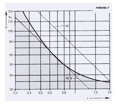
I = switching currentU = switching voltage
