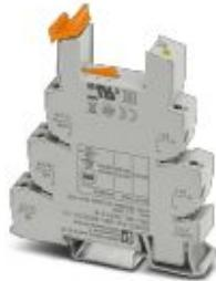
14 mm PLC basic terminal block with screw connection, without relay or solid-state relay, for mounting on DIN rail NS 35/7,5, 2 PDTs, input voltage 60 V DC
