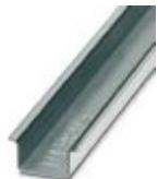
DIN rail, unperforated, Standard profile, width: 35 mm, height: 15 mm, similar to EN 60715, material: Steel, Galvanized, white passivated, length: 2000 mm, color: silver
