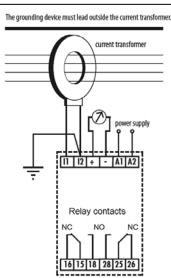
NC = Normally closed. Contact closed when relay de-energised. NO = Normally open. Contact open when relay de-energised.
