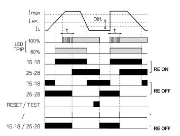
After the connection of the supply voltage to the supply terminals (A1-A2) the green LED goes on. The device is monitoring the value of the leakage current (at terminals I1, I2) by means of external current transformer. If the current value exceeds 60% of the set value the red LED TRIP 60% goes on and relay 1 responds. If the current value exceeds the set value (100%) the red LED TRIP 100% goes on after the delay timing elapses and relay 2 responds. The red LED is flashing during the timing.
