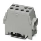
Trunk line branch terminal, Connection method: Screw connection, Number of positions: 1, Cross section: 10 mm² - 35 mm², AWG: 8 - 2, Width: 27 mm, Color: gray, Mounting type: NS 35/7,5, NS 35/15
