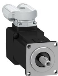
**Servomotor, Lexium BSH, 40mm, 0,39Nm, Passfeder IP54, Multiturn 16P/U, 2xYTEC**
