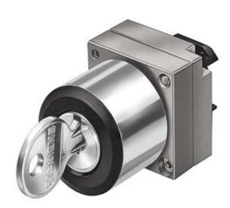
22MM ROUND METAL ACTUATOR: RONIS LOCK WITH 2 KEYS MOMENTARY CONTACT 2 SWITCH POSITIONS O-I LOCK NUMBER SB 30, REMOVE O WITH HOLDER POSSIBLE SPECIAL LOCKS FOR RONIS KEYSWITCHES: SB31, 455, 421
