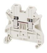
Terminal Blocks, Linergy, feed through, 30A, 600V, screw termination, 2 points, 26AWG to 10AWG, white
