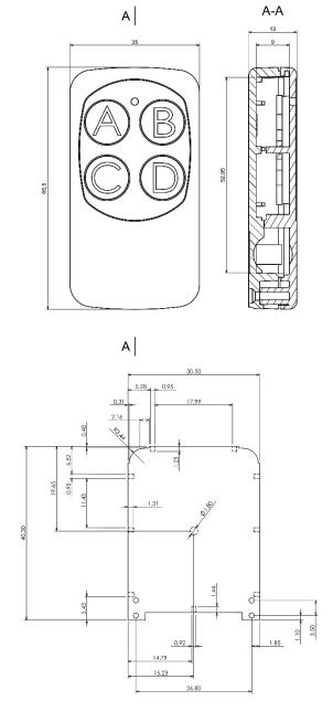
All dimensions are given within +/-0,5mm tolerance
