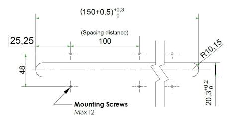
If IP65 is not needed, the amount of **Clip** can be Reduced. And **Spacing distance** can user-defined.
