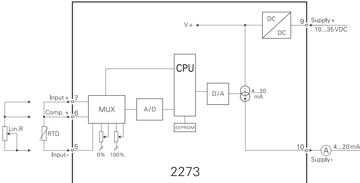
For 2-wire connection, pins 6 and 7 must be short-circuited in the socket.
