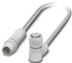
Sensor/Actuator cable, 5-position, PP-EPDM halogen-free, Gray RAL 7035, Plug straight M12, A-coded, on Socket angled M12, A-coded, with 3 LEDs, Cable length: 3 m, Hygienic design, with plastic knurl
