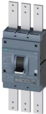
circuit breaker 3VA2 IEC Frame 1250 breaking capacity class C  $I_{cu}=110\text{ kA}$  @ 415 V 3-pole line protection ETU330 LIG  $I_{n}=1250\text{ A}$  overload protection  $I_{r}=500\text{ A}$  ...1250 A short-circuit protection  $I_{i}=15\ldots10 \times I_n$  ground-fault protection  $I_{g}=02\ldots1 \times I_n$   $t_g=01/03\text{s}$  circuit breaker with straight bus connectors extended
