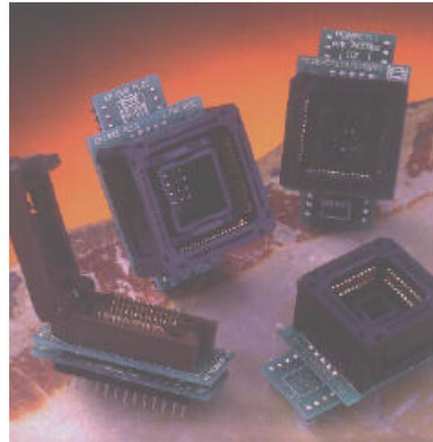
A full range of passive package adapters is available for the LV48 Series of programmers. For most devices up to 48 pins, the module is not device specific, thus reducing the overall number of adapters needed. Package types supported currently include PLCC, PSOP, TSOP, SSOP, SOIC, QFP and BGA. New package types are always being added, and custom made adapters can be developed upon request. To obtain the correct order code please refer to the programmer software or ask your dealer.
